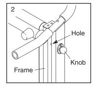
latch pin is fully inserted into the hole.
